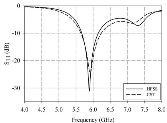
Figure 2 Return loss of the proposed antenna with the ideal setup.
