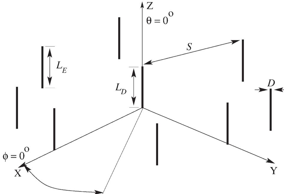
Figure 1 An ideal setup of the proposed monopole antenna with eight parasitic elements.
