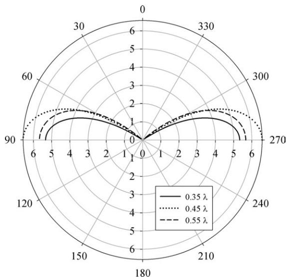
**Figure 3** E-plane gain patterns in dB at 5.9 GHz with varying spacing (*S*).
