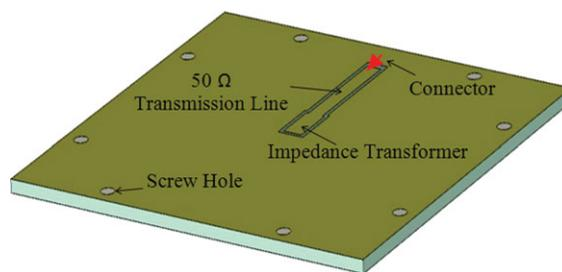
**Figure 5** Feed network configuration. [Color figure can be viewed in the online issue, which is available at wileyonlinelibrary.com.]
