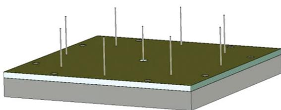
Figure 7 Proposed fully integrated antenna (i.e., combination of the ideal antenna, the feed network board, and a metal base). [Color figure can be viewed in the online issue, which is available at wileyonlinelibrary.com.]
