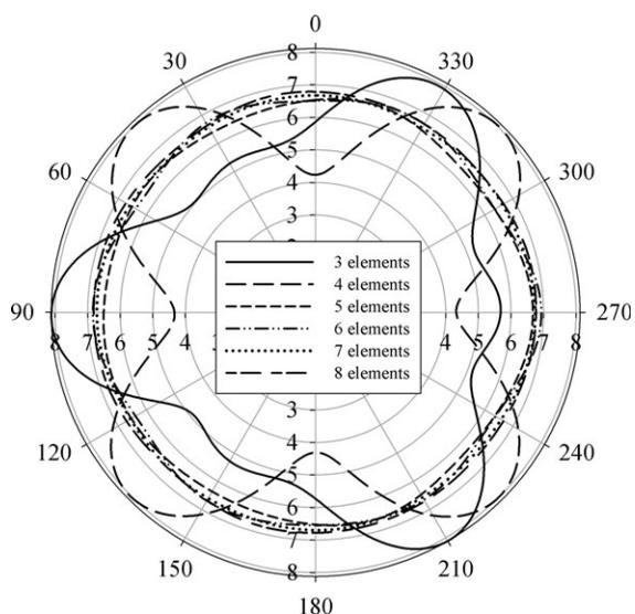
**Figure 4** H-plane gain patterns in dB at 5.9 GHz with different number of parasitic elements.
