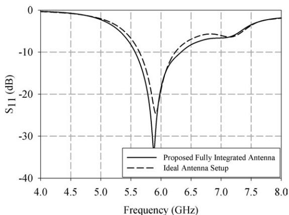
Figure 8 Return loss of both ideal and fully integrated antenna.
