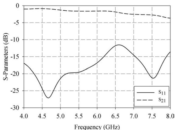
Figure 6 S-parameters results of the quarter-wave transformer.
