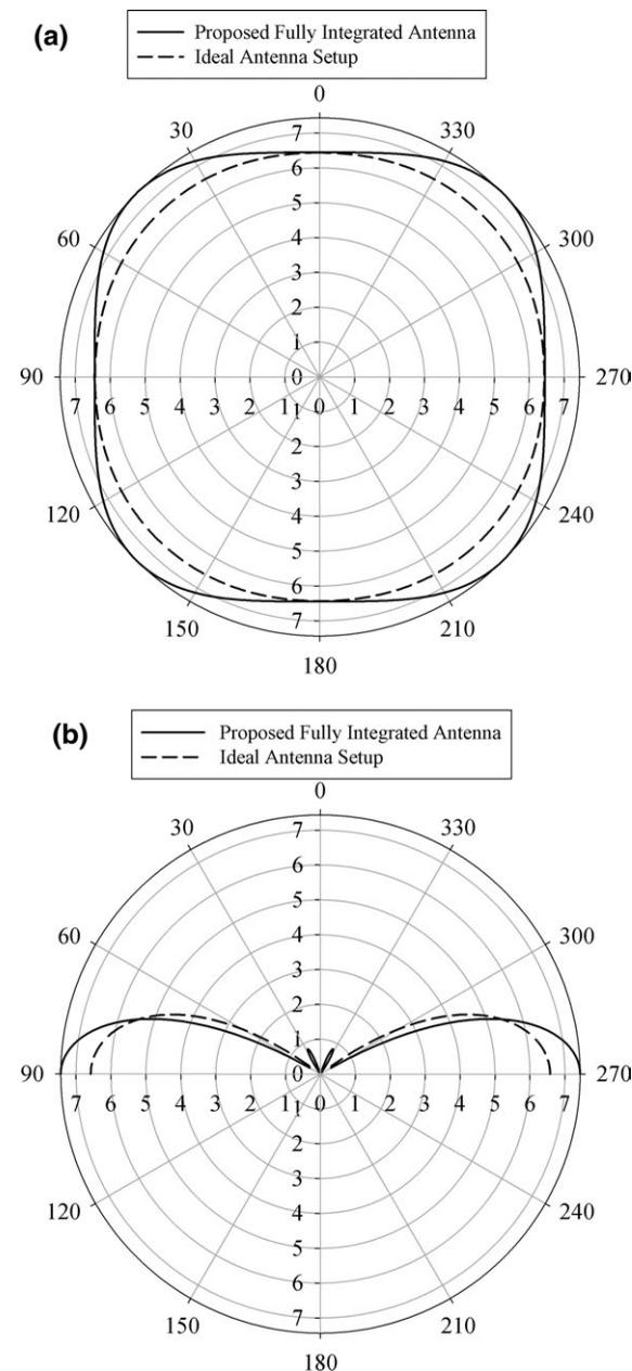
Figure 9 Evaluated antenna gain pattern in dB for both ideal and fully integrated antennas at 5.9 GHz: (a) *H*-plane and (b) *E*-plane.
