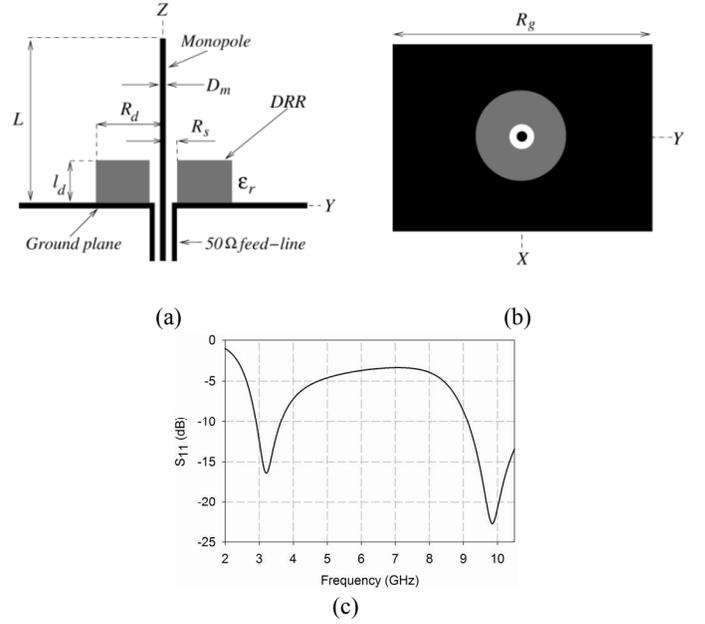
Fig. 2. (a) Cross-sectional view of the broadband monopole-DRR antenna; (b) its top view; and (c) the simulated reflection coefficient ( $S_{11}$ ) of the monopole wire antenna without the DRR showing narrow impedance bandwidth at 3.2 GHz.
