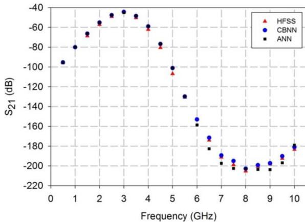
Fig. 8. Insertion loss ( $S_{21}$ ) results of the WG using HFSS, proposed CBNN, and ANN.
