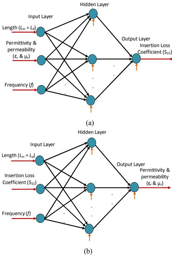
Fig. 6. (a) ANN model for antenna example; and (b) its selected CBNN model.
