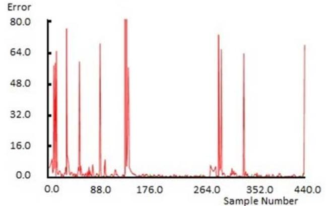
Fig. 7. Graph showing percentage error after training using Huber-Quasi Newton algorithm.
