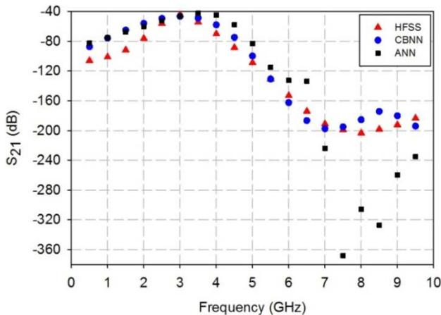
Fig. 9. Simulated S-parameter transmission coefficient ( $S_{21}$ ) of the waveguide example using HFSS, proposed two-stage CBNN and ANN.
