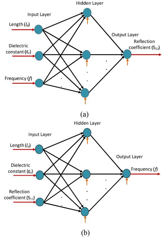
Fig. 4. (a) ANN model for antenna example; and (b) its selected CBNN model.
