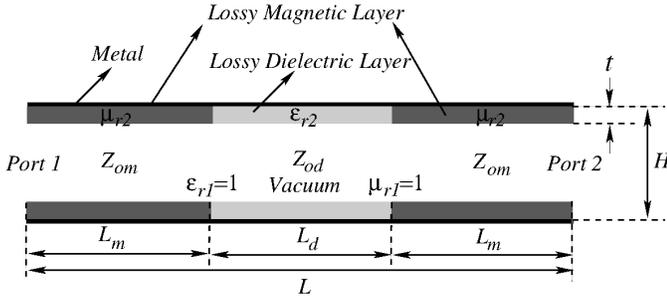
Fig. 3. Side cross-section view of the WG coated with three segments of lossy materials as an example. The stepped variations consist of the following order: lossy magnetic-dielectric-magnetic along the WG length ( $L$ ).
