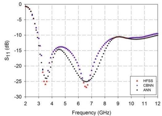
Fig. 5. Reflection coefficient ( $S_{11}$ ) results of the monopole DRR antenna using HFSS, proposed CBNN, and ANN.
