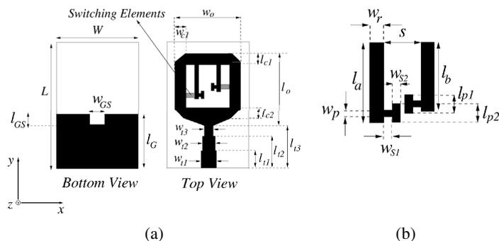
Fig. 1. Physical structure of the proposed SWB antenna (a) top and bottom view; and (b) its bandstop resonators (zoom view).
