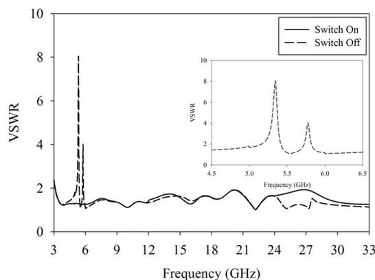
Fig. 4. Simulated VSWR response against frequency of the proposed antenna with switch on/off.
