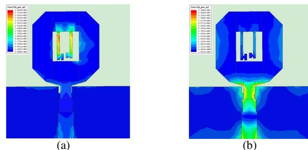
Fig. 2. Simulated current distributions at: (a) the lower WLAN notch frequency (5.3 GHz); and (b) out of the rejection bands (8 GHz).
