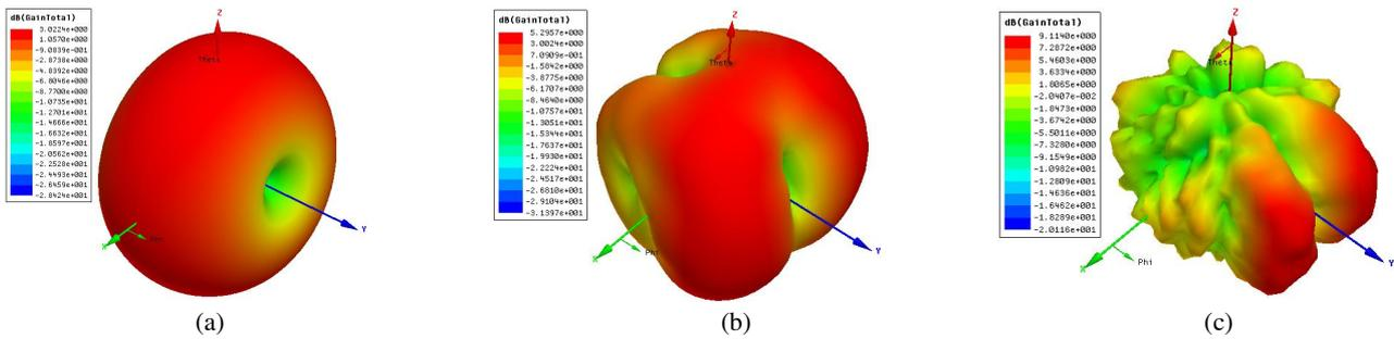
Fig. 5. Simulated 3D far-field radiation pattern of the proposed antenna at: (a) 4 GHz; (b) 9 GHz; and (c) 15 GHz.
