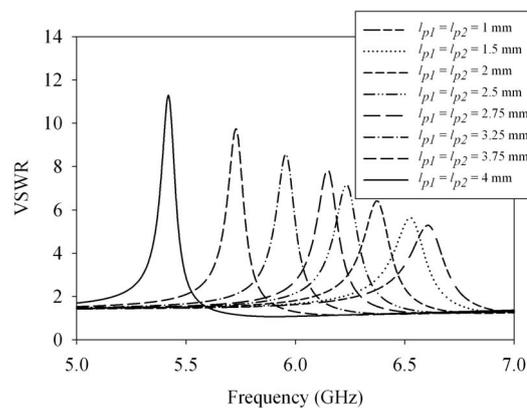
Fig. 3. Simulated VSWR response against frequency by varying the bandstop resonator's length of Fig. 1(b).
