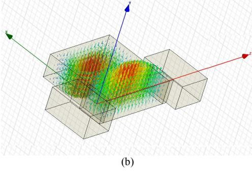
Fig.2 (a) Electric field distribution of TE<sub>102</sub> mode and (b) Electric field distribution of TE<sub>201</sub> mode.
