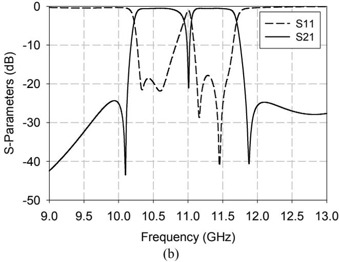
Fig. 4. (a) Top view configuration of the proposed three-cavity dual-band dual-mode SIW filter and (b) its simulated frequency characteristics.
