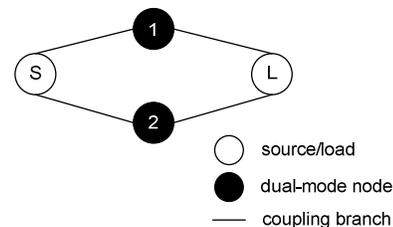
Fig.1. Coupling topology of a dual-mode SIW cavity.
