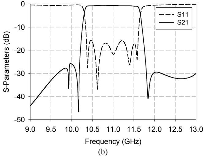
Fig.3. (a) Top view configuration of the three-cavity bandpass dual-mode SIW filter and (b) its simulated frequency characteristics.
