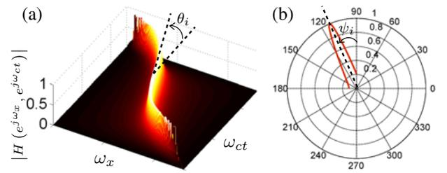
Fig. 3: Example (a) magnitude frequency response and (b) array factor of a first order 2-D IIR digital beam filter.
