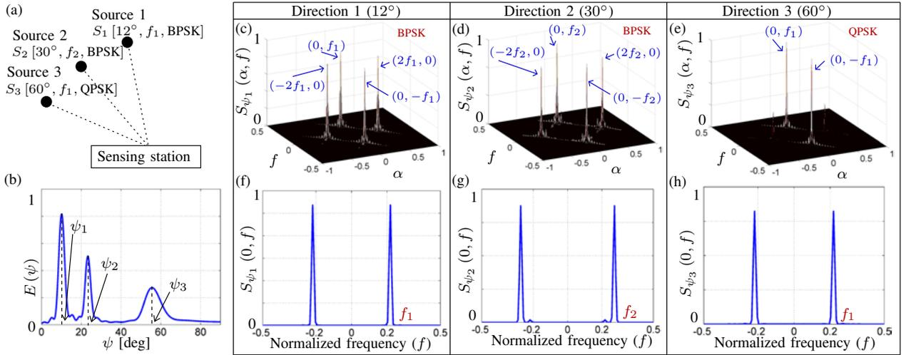
Fig. 4: (a) Source distribution, (b) spatial energy distribution  $E(\psi)$  and (c)-(h) various feature detection outputs corresponding to the simulation scenario 1.
