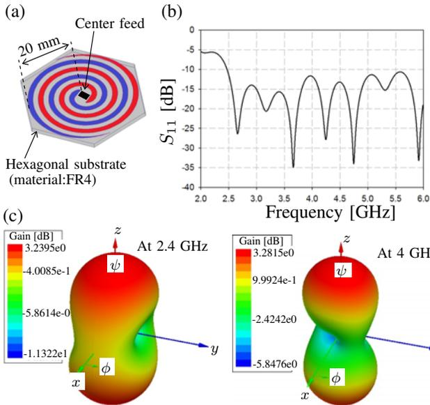
Fig. 2: (a) Structure, (b) scattering parameter  $S_{11}$  and (c) far-field radiation pattern of the proposed Archimedean spiral antenna. Full-wave simulations are from Ansoft HFSS computational electromagnetic software.
