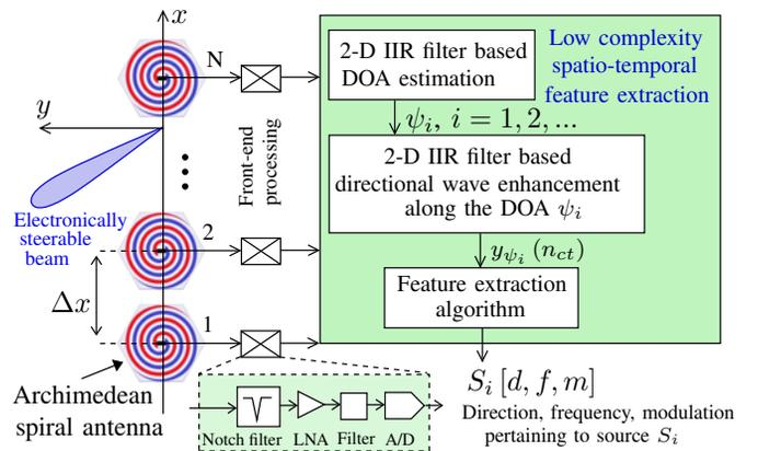
Fig. 1: Overview of the proposed 2-D IIR digital beam filter based directional feature extraction system employing a ULA of Archimedean spiral antennas.
