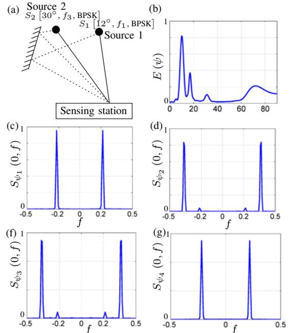
Fig. 5: (a) Source distribution, (b) spatial energy distribution  $E(\psi)$  and (c)-(f) SCF at  $\alpha = 0$  corresponding to simulation scenario 2.
