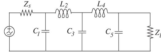
**Figure 6** Circuit prototype of 5-element open-circuited stub LPF.
