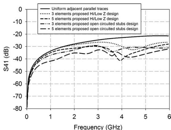
**Figure 10** Far-end crosstalk in PCB traces using the proposed configurations.
