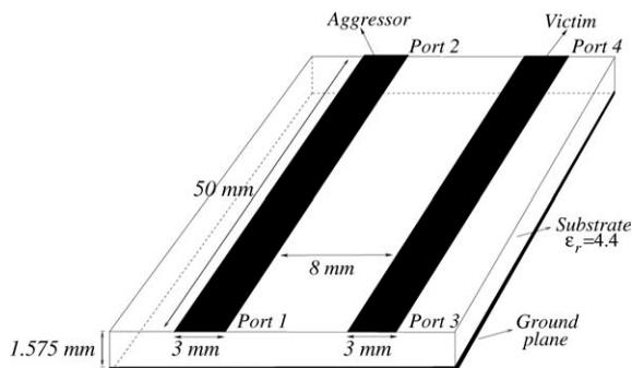
Figure 1 PCB structure with two uniform adjacent traces.
