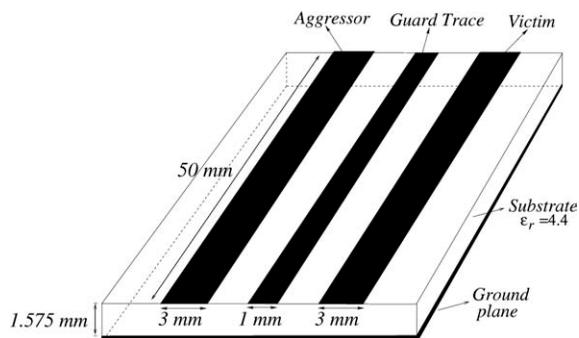
Figure 2 PCB structure with a guard trace between two uniform adjacent traces.
