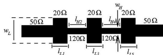
Figure 4 5-Element stepped impedance LPF design.
