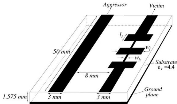
**Figure 5** PCB structure of the proposed stepped impedance configuration with five elements.
