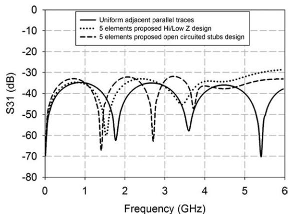
**Figure 11** Comparison between the proposed configurations and the uniform trace configuration for the near-end crosstalk.
