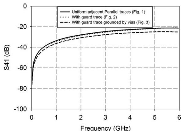
**Figure 9** Comparison of far-end crosstalk in adjacent PCB traces using a guard trace and a guard trace grounded with vias.
