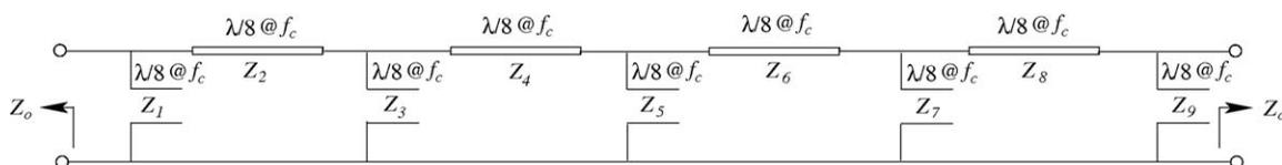
**Figure 7** A distributed circuit model of a 5-element open-circuited stub LPF design.
