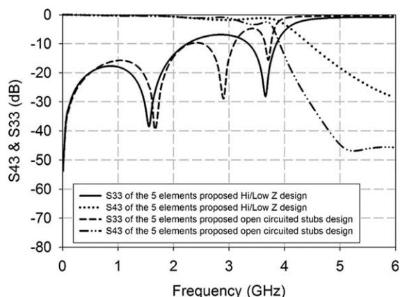
**Figure 12** LPF frequency characteristics for both proposed configurations.
