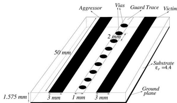
Figure 3 PCB structure with a guard trace grounded with vias between two uniform adjacent traces.
