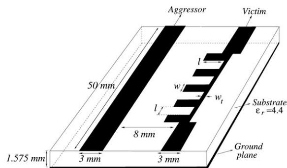
**Figure 8** PCB structure of an open-circuited stub configuration with five elements.
