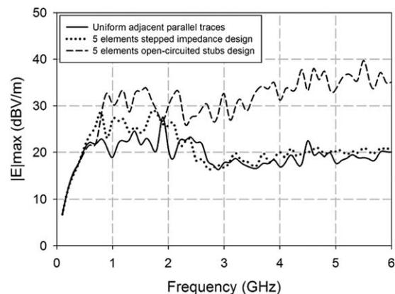
**Figure 13** Magnitude of radiated electric field from the proposed PCB configurations.
