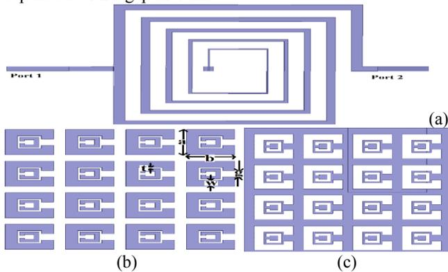
Fig. 3. (a) Layout of the spiral inductor with two ports (turns=3, inner dimension=60 $\mu\text{m} \times 80 \mu\text{m}$ , overall dimension=
