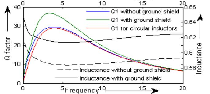
Fig. 4. Simulated  $Q$  factors of the inductors at port 1 (i.e.  $Q_1$ ) with and without the two layer ground shield.
