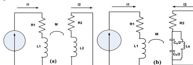
Fig. 1. Equivalent circuit model illustrating the effect of negative and positive mutual coupling in (a) Solid Ground Shield (b) CSRR-SRR patterned ground shield (exhibiting left-handed behavior).
