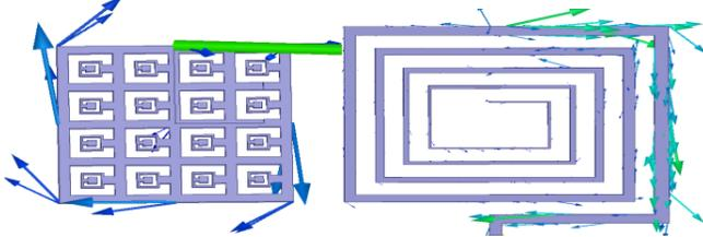
Fig. 2. Simulated surface current vector on the ground shield and inductor showing that the current direction in both is same.
