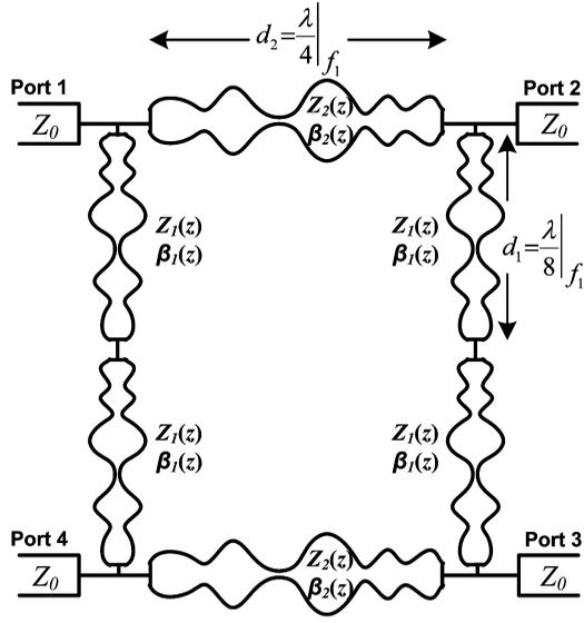
Figure 1. Schematic diagram for proposed NTL multi-band BLC.
