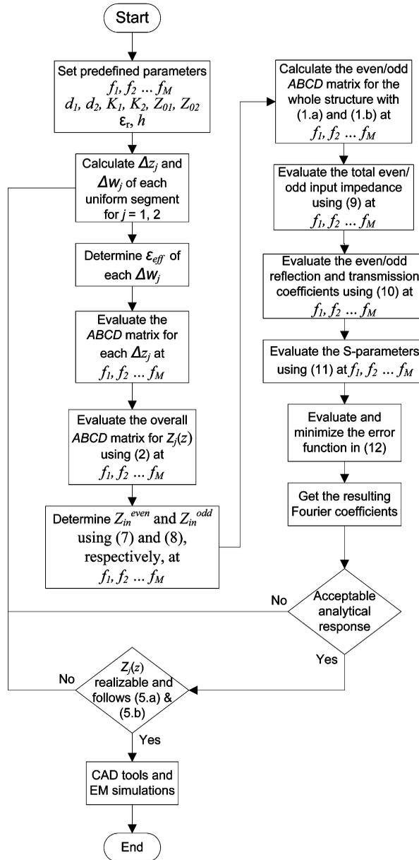
Figure 3. Flowchart demonstrating general design procedure of multi-band non-uniform BLC.
