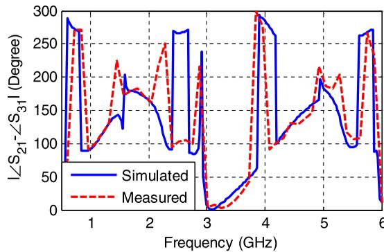
**Figure 10.** Simulated and measured phase difference between  $S_{21}$  and  $S_{31}$ .
