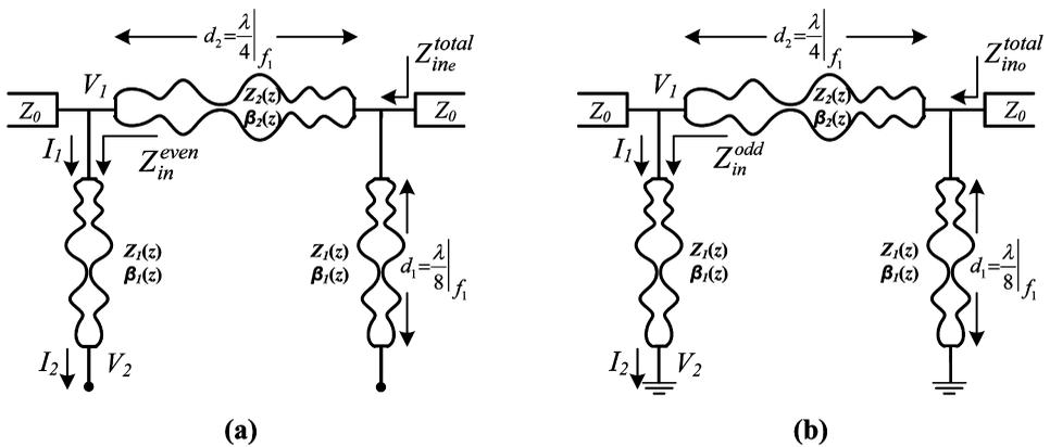
Figure 2. Proposed non-uniform BLC: (a) even-mode circuit and (b) odd-mode circuit.
