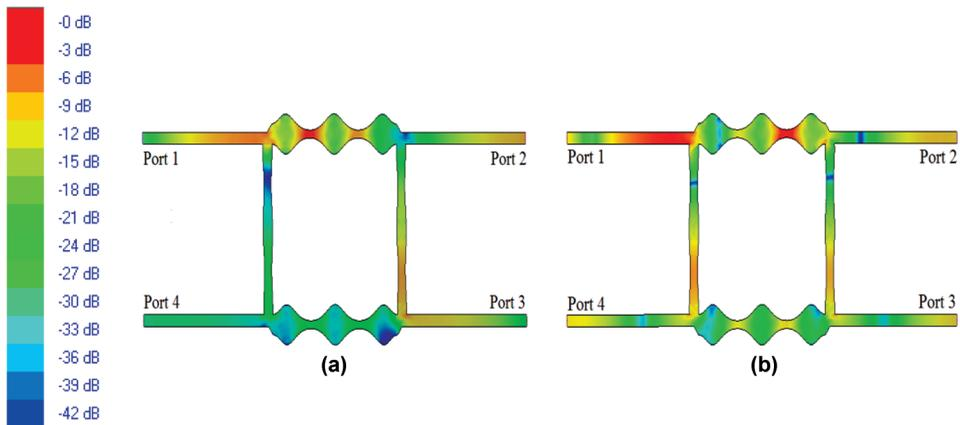
**Figure 7.** Current distribution of dual-band 3-dB  $90^\circ$  BLC: (a) in-band frequency (0.86 GHz) and (b) out-of-band frequency (1.5 GHz).
