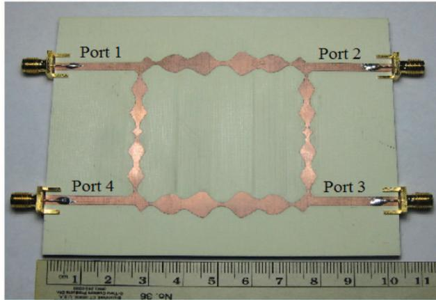
**Figure 8.** Photograph of fabricated triple-band 3-dB  $90^\circ$  BLC.
