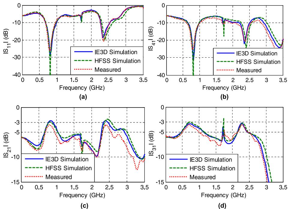
**Figure 5.** Simulation and measurement results for dual-band 3-dB 90° BLC: (a) input port matching parameter ( $S_{11}$ ) (b) isolation parameter ( $S_{41}$ ), (c) transmission parameter ( $S_{21}$ ), and (d) transmission parameter ( $S_{31}$ ).
