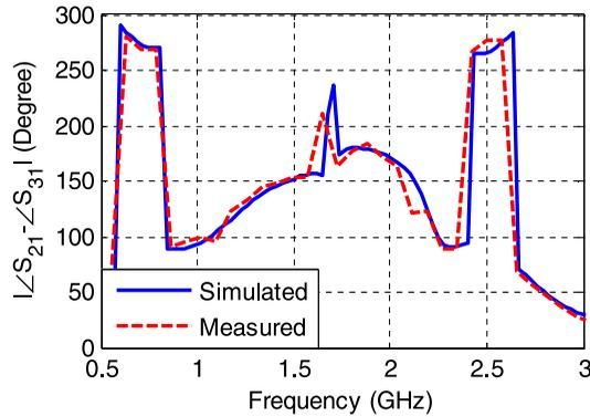
**Figure 6.** Simulated and measured phase difference between  $S_{21}$  and  $S_{31}$ .
