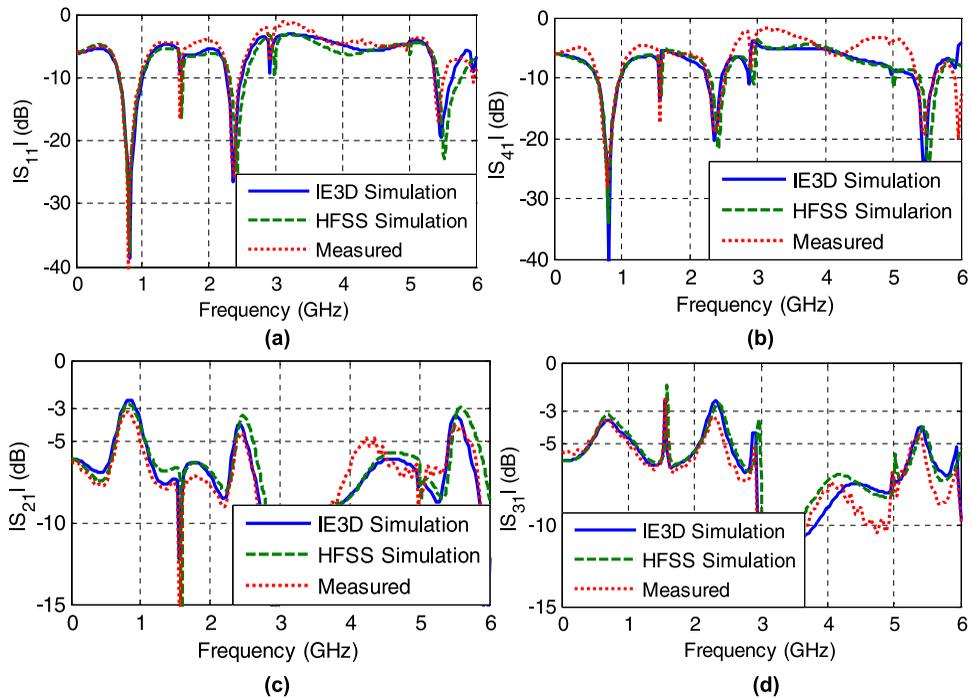
**Figure 9.** Simulation and measured results for triple-band 3-dB  $90^\circ$  BLC: (a) input port matching parameter ( $S_{11}$ ), (b) isolation parameter ( $S_{41}$ ), (c) transmission parameter ( $S_{21}$ ), and (d) transmission parameter ( $S_{31}$ ).
