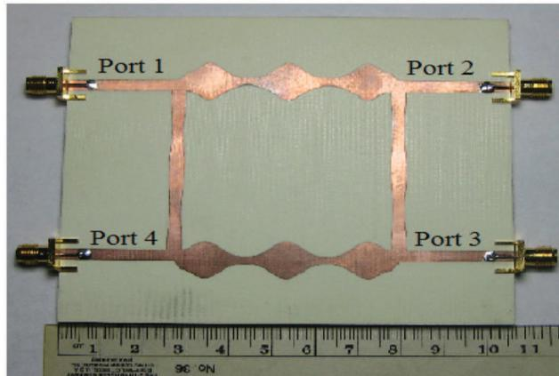
**Figure 4.** Photograph of fabricated dual-band 3-dB 90° BLC.
