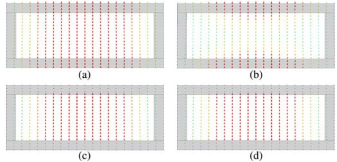
Fig. 5. Electric field distribution of the  $TE_{10}$  mode at a frequency below  $f_c$  (at 3 GHz) and above  $f_c$  (at 6 GHz) for a rectangular WG coated with (a) and (b) uniform magnetic and (c) and (d) uniform dielectric material.
