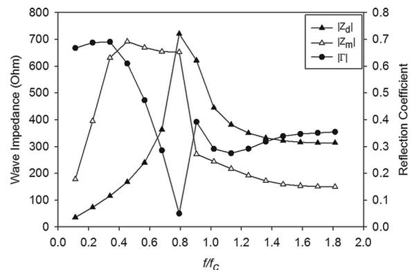
Fig. 6. Magnitude of the wave impedance for a WG coated with a uniform lossy magnetic ( $Z_m$ ), a uniform lossy dielectric ( $Z_d$ ), and the reflection coefficient magnitude ( $\Gamma$ ) versus normalized frequency.
